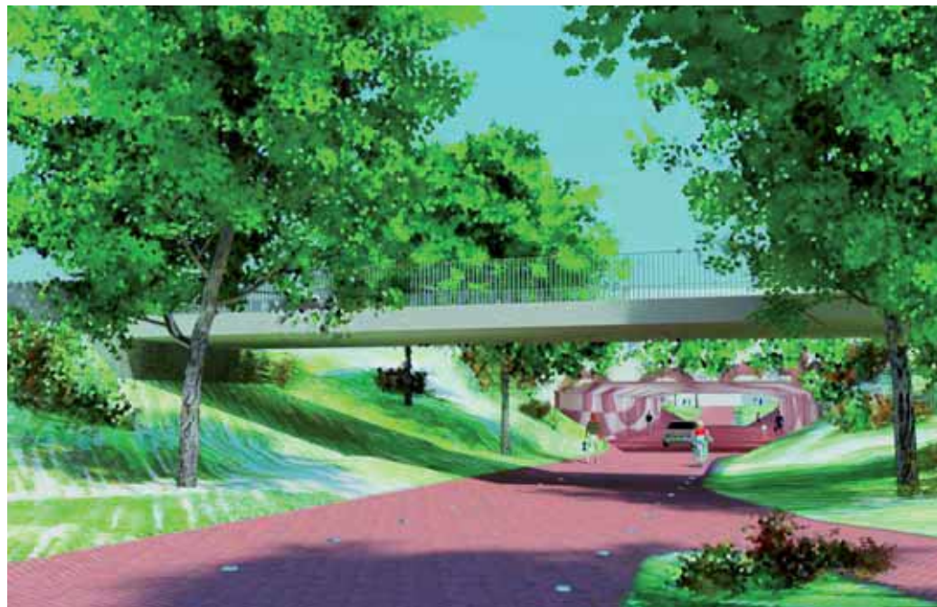
Intervention: smoothing out the edges of the underpass, integrating the road into the Sidelinge park and creating shared space
